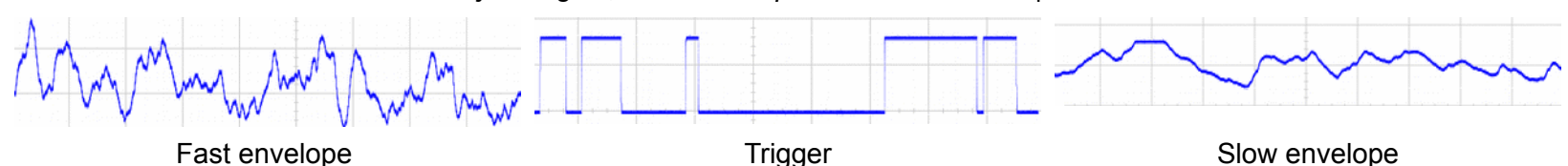
Env Out jack signal, at the three positions of the Fast | Slow switch
